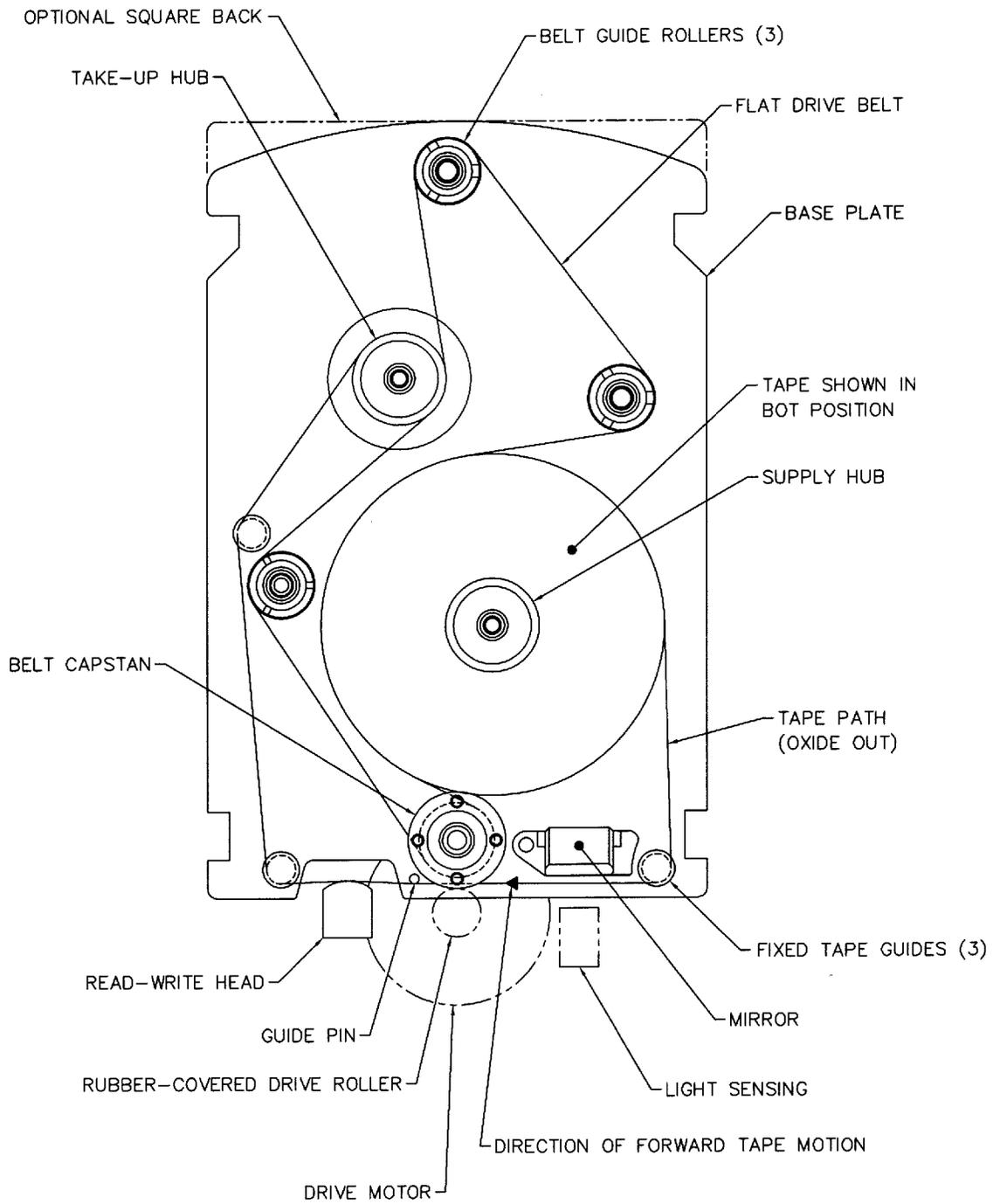
FIG. 1 - CARTRIDGE CONFIGURATION
